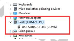
3.Come with USB programming cable port is USB-SERIAL CH340 (COM?)
